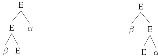
(a) Valid tree when prio(\langle E, \beta E \rangle) > prio(\langle E, E \alpha \rangle) (b) Valid tree when prio(\langle E, E \alpha \rangle) > prio(\langle E, \beta E \rangle)
